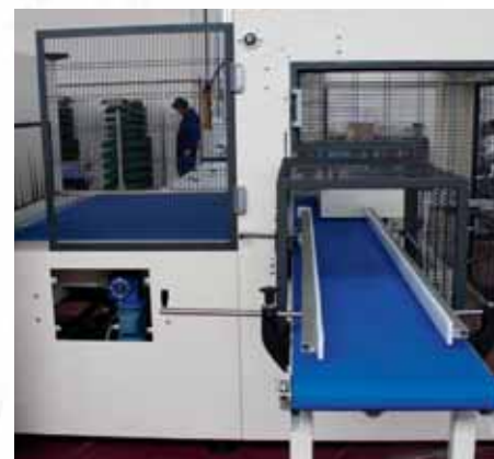
The machine can be equipped with in line conveyor; 90° conveyor with pusher for higher speed, and for automatic multipack forming.
