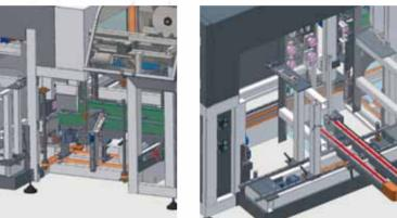
All adjustments are motorized. Mouvements on Hiwin linear guides.
