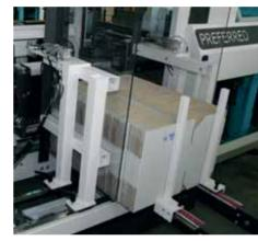
Easy access and load of cartons in the stock-magazine unit.
