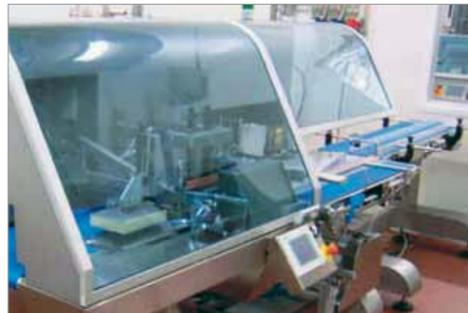
*The machine can use, neutral or pre-printed film, center folded or flat film (as POLIOLEFIN FILM, POLYPROPYLENE, BOPP, PE, Barrier Film). To create also map packaging or vacuum packaging with hermetic seals.*
